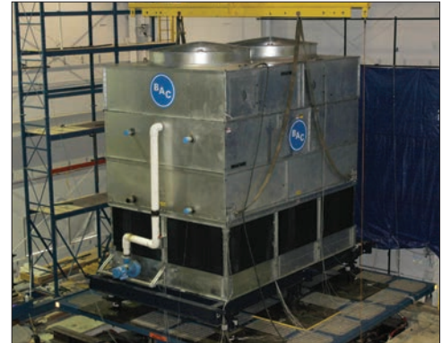
Shake Table Tested up to 3.1g
