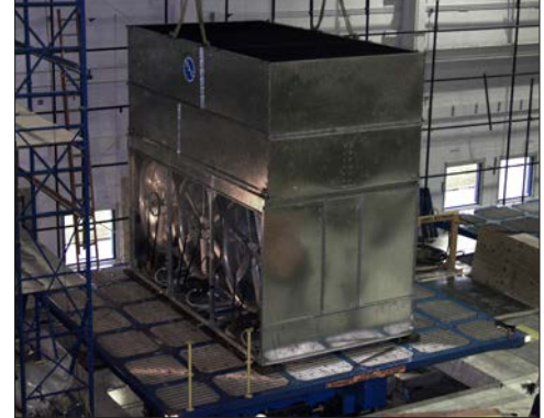
Shake Table Testing
